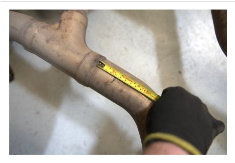
We recomend removing the original exhaust from the car before cutting.
